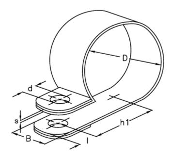
$\begin{array}{ll} d & = 5.3 \\ \text{Diameter D} = 11 \\ \text{h1} & = 12.3 \\ \text{I} & = 5.0 \\ \text{s} & = 0.5 \\ \text{Width B} & = 12 \\ \end{array}$
